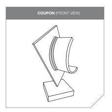
Coupon's material: Carbon Steel ASTM A 36 thickness 6 mm
